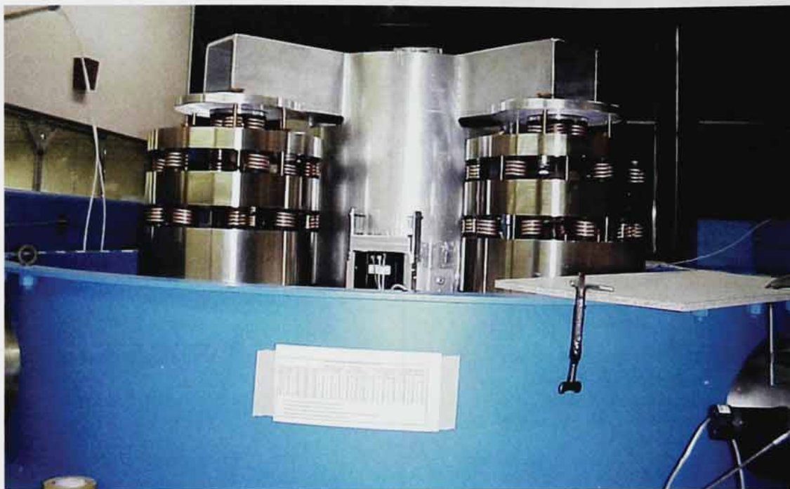
FIGURE 5. LIGO'S SEISMIC ISOLATION SYSTEM consists of four layers of masses and springs. Each of the coil springs seen here is made by lining the inside of a straight metal tube with rubbery damping material and then filling the lined tube with a line of metal slugs strung on a rubber core. The tube is then coiled and sealed.
