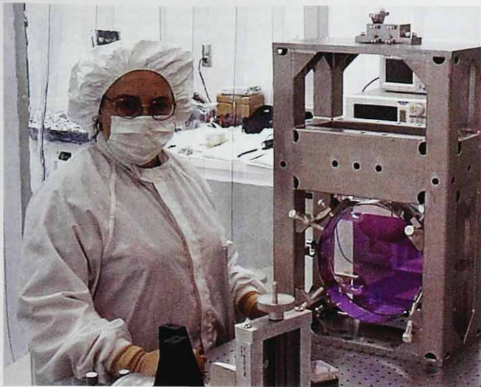
FIGURE 6. A LIGO MIRROR, 25 cm in diameter and 10 cm thick, is made of ultrapure fused silica. Its purple coating is a highly reflective multilayer stack of dielectric materials. Absorption and scattering losses must not exceed a few parts per million.
