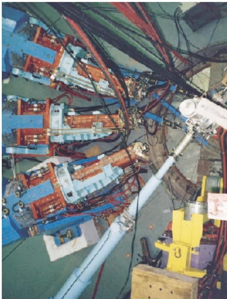
FIGURE 7.7 The Out-of-Plane-Spectrometer (OOPS) at the Bates accelerator is used to study polarization phenomena in nuclei. The four spectrometers allow positioning out of the reaction plane, which is important for the analysis of polarization variables. (Courtesy MIT Bates Linear Accelerator Center.)
