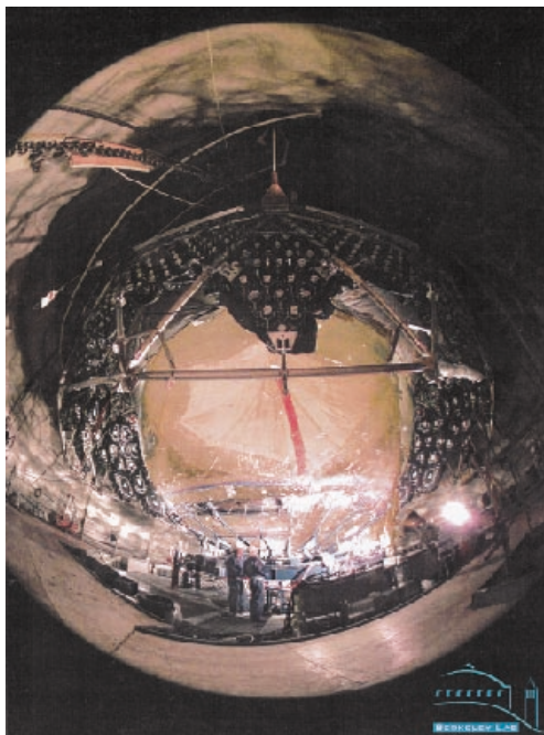
FIGURE 5.1.2 The Sudbury Neutrino Observatory, viewed through a fisheye lens, just before completion. The inner spherical acrylic vessel will isolate SNO's 1,000 tons of heavy water from the surrounding ordinary water that will fill the entire cavity when the detector is operating. The concentric darker structure is the array of 9,500 photomultiplier tubes (PMTs) nearing completion. The PMTs view light produced in the inner water volumes and are temporarily covered with removable shields to maintain low levels of surface contamination. The PMT array is 18 m in diameter. The detector is located 2,000 m underground in the INCO mine in Sudbury, Ontario, Canada. (Courtesy of Lawrence Berkeley National Laboratory.)
