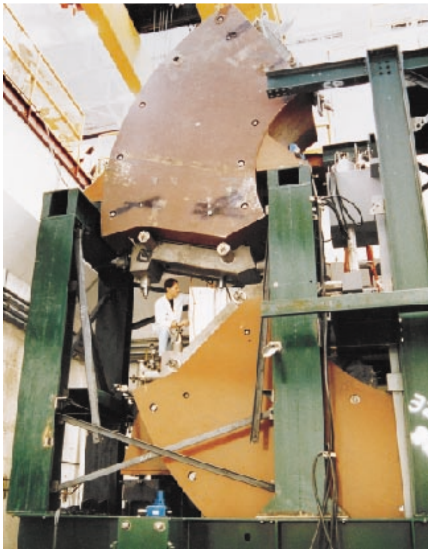
FIGURE 7.5 The superconducting magnetic spectrograph S800 at Michigan State University. The target for the nuclear reactions is at the bottom left of the spectrometer structure. Reaction products from nuclear collisions, induced by beams of shortlived nuclei (radioactive beams) are selected and bent upwards by powerful superconducting magnets onto the focal-plane detector system mounted on the top of the spectrograph. (Courtesy MSU.)
