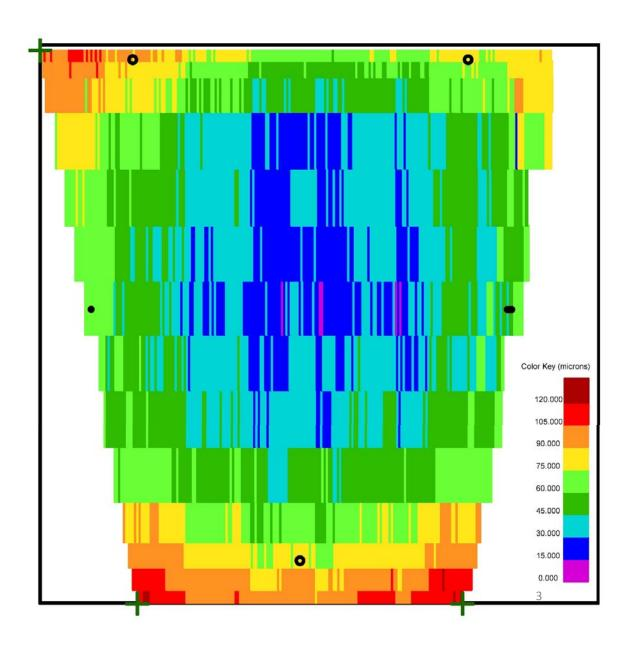
Height differences from best fit flat plane. Fit parameters = rotation about X and Y axis. X slope =  $-2.87 \times 10^{-5}$
