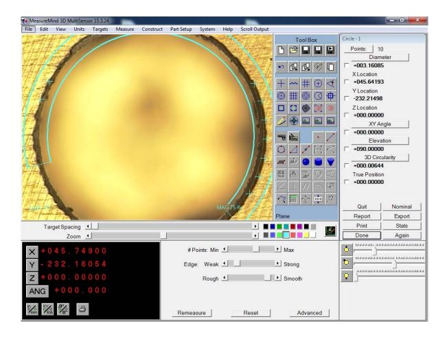
Typical OGP measurement screen. This shows feature fitting – user defines 3 points on the circle, the machine then finds several points and fits a circle. Ignore values here, image was taken before part setup was complete.
