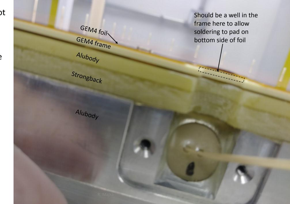
I-G4-020 – frame us machined properly. The wells for soldering to the bottom HV pads are present.
