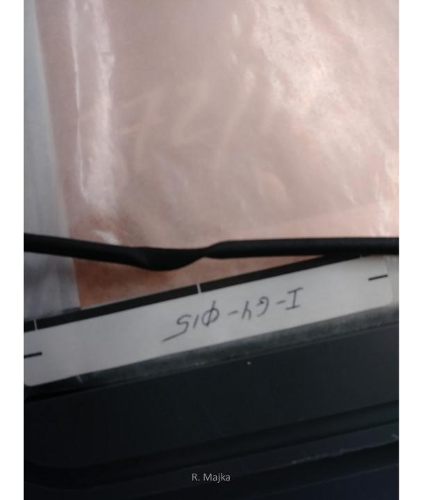
I-G4-019 – frame not machined properly. The wells for soldering to the bottom HV pads are missing.
