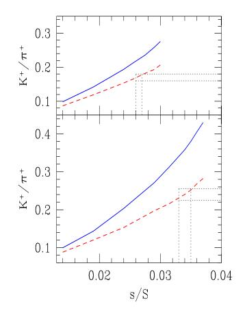
$K^+/\pi^+$  ratio as function of attained specific strangeness at freezeout, s/S. Solid lines bare yields, dashed lines after all weak decays have diluted the pion yields. Top for RHIC and bottom for LHC physics environment. An increase by about 40% is predicted from  $K^+/\pi^+ = 0.17$  at RHIC to  $K^+/\pi^+ = 0.24$  at LHC. If LHC is subject to donut-expansion, increase more significant.
