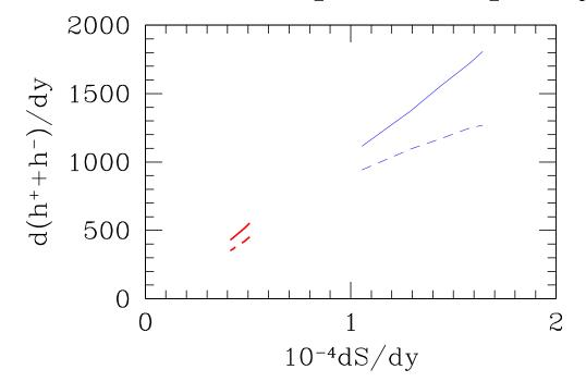
The yield of charged hadrons  $d(h^- + h^+)/dy$  for different values of dS/dy. Solid lines: after all weak decays, dashed lines: before weak decays. Left domain for RHIC and right domain for LHC - defined at E/b = 40,412 GeV respectively,obtained not as fit to data but assuming E/TS = 0.78, baryon conservation etc. See: hep-ph/0506140 and Eur. Phys. J. C (2005) -02414-7 by JR and JL "Soft hadron ratios at LHC"
