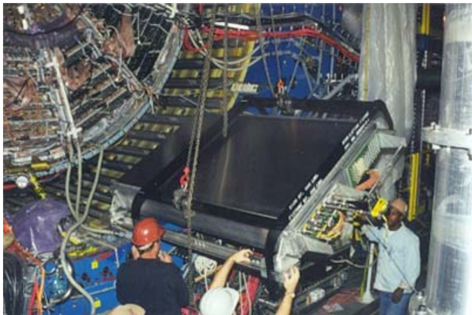
Figure 2.18: Installation of the RICH detector into the STAR experimental set-up. The detector is shown housed in the aluminum safety box. A large frame is seen attached to the detector for the purposes of installation and is not present during data taking.
