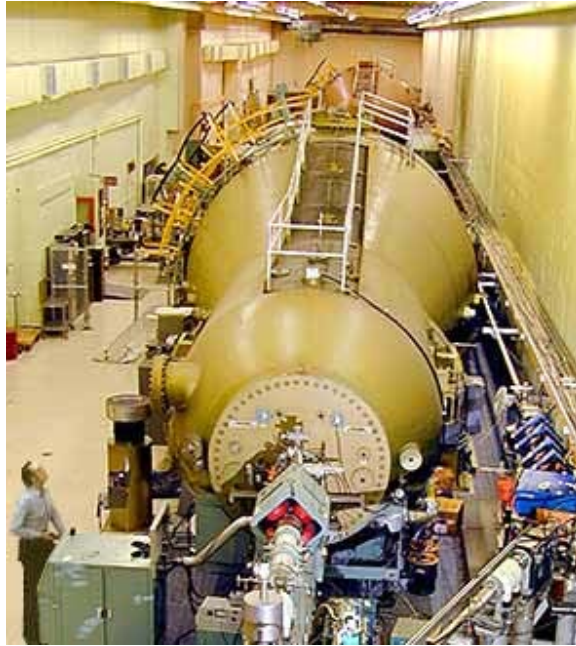
Figure 2.2: Tandem Van de Graaff at Brookhaven National Laboratory.
