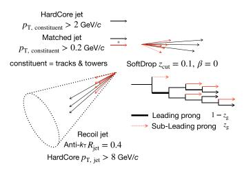
FIG. 2. Visualization of the SoftDrop declustering step applied on a recoil jet resulting in the selection of the leading and subleading prongs.
