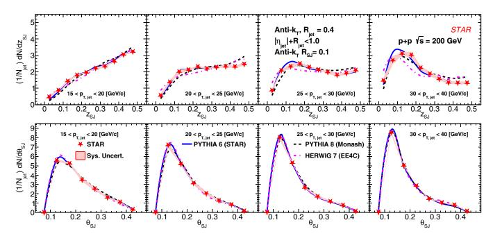
FIG. 6. Distributions of fully unfolded two-subjet observables  $z_{SJ}$  in the top panels and  $\theta_{SJ}$  in the bottom panels for inclusive jets in p+p collisions shown in the red star markers, compared to leading-order MC event generators PYTHIA 8 (black), PYTHIA 6 (blue), and Herwig 7 (magenta) for low- $p_T$  jets on the left to high- $p_T$  jets on the right. The shaded red regions represent the systematic uncertainties in the data points.
